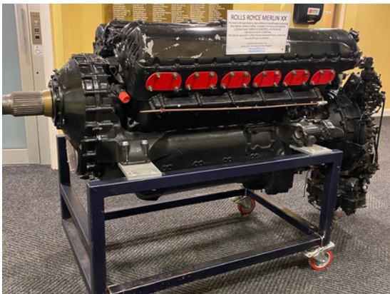
Above: A Rolls Royce Merlin XX Engine (fitted in Beaufighters, Hurricanes, Lancasters and Spitfires.)
